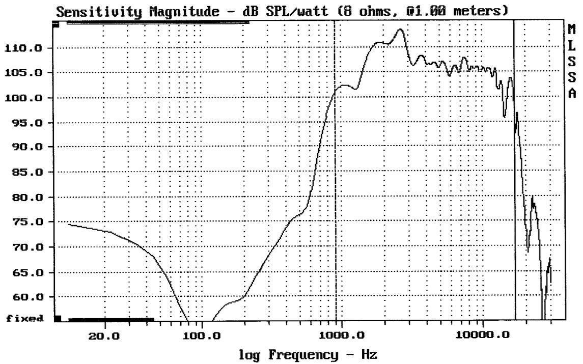
Level (899:16801 Hz) = 107.40 dB SPL/watt (8 ohms, @1.00 meters)
