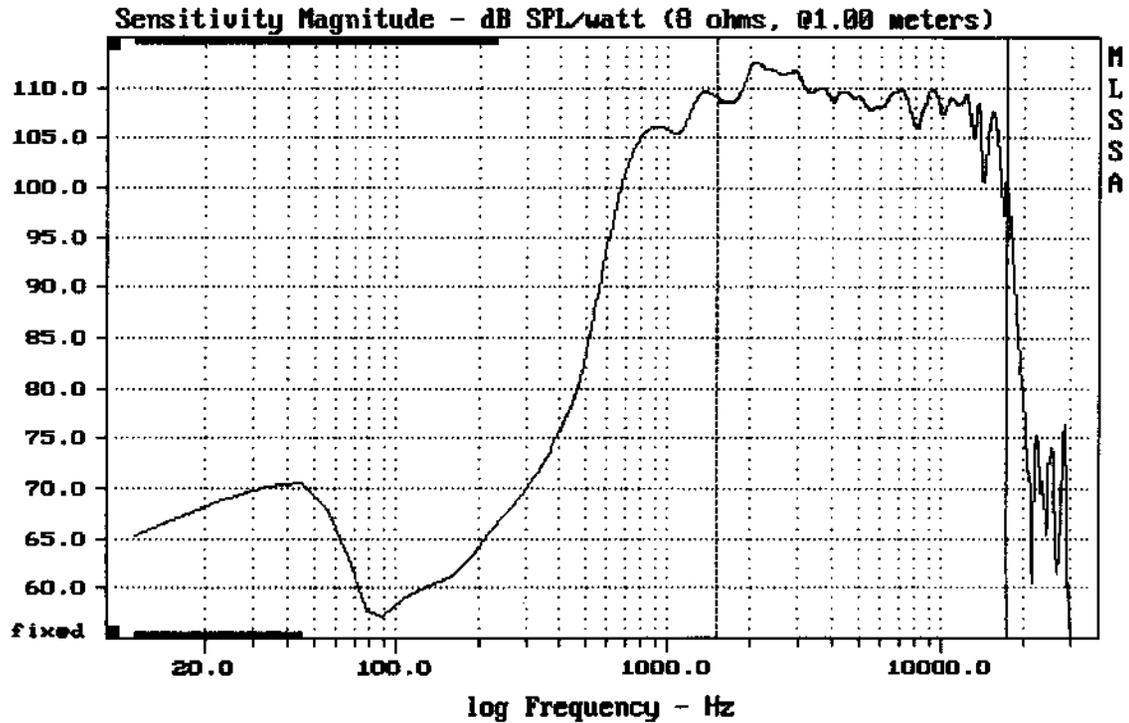
Level (1498:17500 Hz) = 109.33 dB SPL/watt (8 ohms, @1.00 meters)
